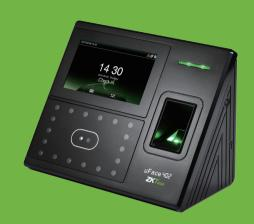
uFace402 Facial multi-biometric time & attendance and access control terminal supports up to 3,000 face templates, 4,000 fingerprint templates and 10,000 cards (optional). With ZKTeco latest hardware platfrom and algorithm, it offers brand new Uland user-friendly operation interface to provide smooth user experience. With advanced face algorithm and multi-biometric verification technology, the terminal's security level of verification is significantly enhanced.
